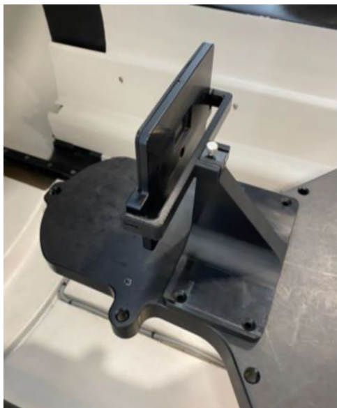
FIGURE 15 Setup for start shot measurement.
