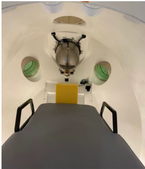
FIGURE 10 Collimator collision test using a soft object on the table.
