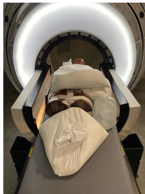
FIGURE 16 Setup for tabletop sag measurement.
