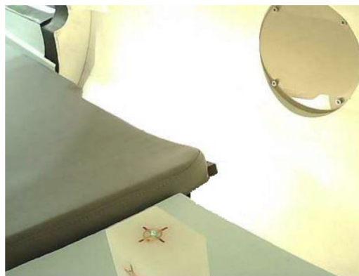
FIGURE 21 Coincidence of the laser (green) and the anterior marker for positioning/repositioning accuracy check using kV imaging. kV, kilovoltage.
