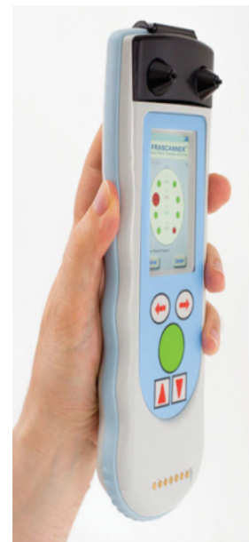
FIGURE 2: The infrascanner intracranial haematoma detector, model 2000. Courtesy of Infrascan Handheld brain diagnostics.
