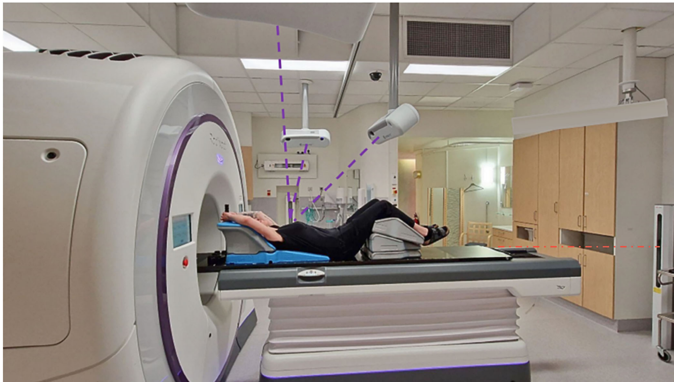
FIGURE 1 The SGRT system setup for the tomotherapy system and a healthy volunteer positioned on the couch for SGRT measurements. A laser projector device (red dashed line) is located at the end of the couch to track the position of the couch in real-time and communicate with the main (middle) camera. The SGRT cameras (purple dashed lines) are at 120^\circ angles from each other, tilted 36^\circ , and mounted 1.10 m in height (from treatment iso-center) and 1.70 m outside the treatment iso-center. SGRT, surface guided radiotherapy.
